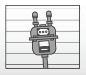
The natural gas meter is starting to tilt or shift.
